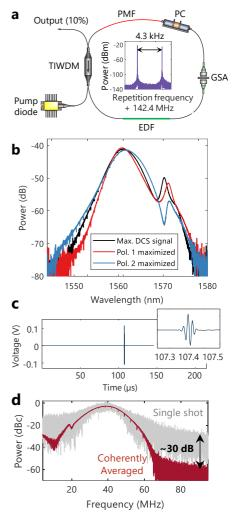
**Fig. 1. (a)** Experimental setup, **(b)** Optical spectra, **(c)** DCS interferogram, **(d)** Dual-comb spectra with HCN in the beam path in 230  $\mu$ s and averaged (200 ms). See text for details.
