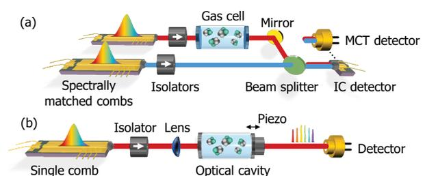
Fig. 1. Two topologies for chip-based, mode-resolved MWIR OFC spectroscopy: (a) Dual-comb spectrometer with a mercury-cadmium-telluride (MCT) or interband cascade (IC) detector. (b) Vernier spectrometer with cavity enhancement.
