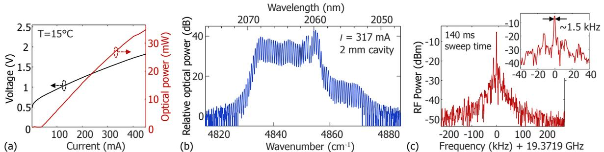
Fig. 1. Device characterization. (a) Light-current-voltage characteristics. Frequency comb generation occurs between 250 mA and the maximum current (450 mA) with more than 35 mW of optical power. (b) Example optical spectrum in a frequency comb regime. (c) The corresponding microwave intermode beat note 3 dB linewidth is  $\sim 1.5$  kHz.
