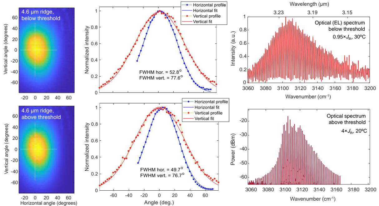
Fig. 1. Full far-field profiles (left), horizontal and vertical beam cross-sections (center), and emission spectra (right), for a 4.6-  $\mu\text{m}$ -wide ridge measured below (top row), and above (bottom row) threshold. The optical spectra were measured by a Fourier transform spectrometer (FTIR), and the horizontal angle is limited on the negative side due to mechanical constraints of the stage assembly.
