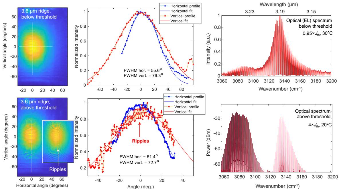
Fig. 2. Full far-field profiles (left), horizontal and vertical beam cross-sections (center), and emission spectra (right) for a  $3.6\text{-}\mu\text{m}$ -wide ridge measured below (top row), and above (bottom row) threshold.
